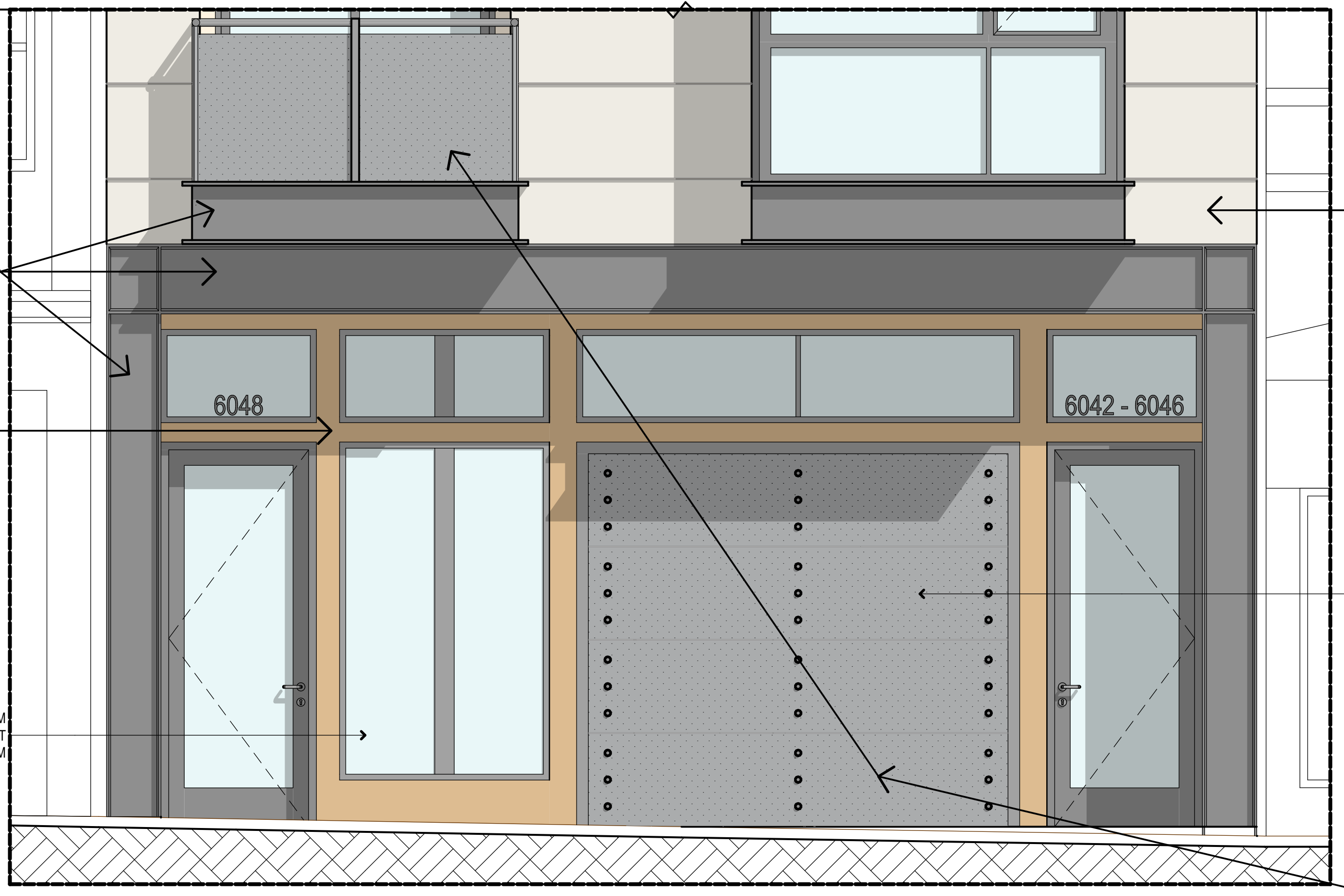
2 GROUND FLOOR FACADE ALL DIMENSIONS FROM FINISH TO FINISH, U.O.N. SCALE: 1/2" = 1'-0"
