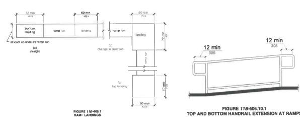
TOP AND BOTTOM HANDRAIL EXTENSION AT RAMPS
